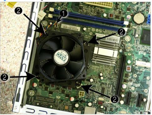
Figure 2-46 Removing the heat sink
